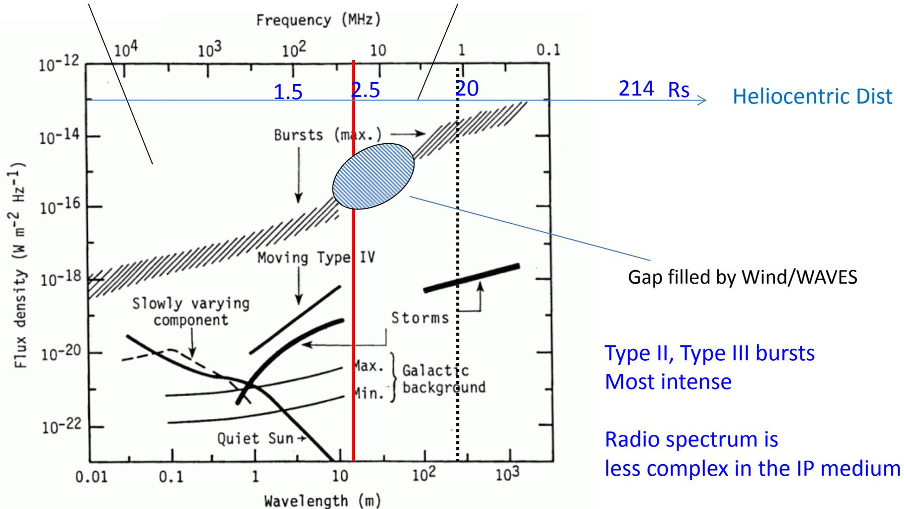
Flux densities of the quiet Sun (at sunspot minimum) and of large solar bursts of several types. Also shown is the range of the galactic background flux ( $20^\circ$  beamwidth is assumed).
